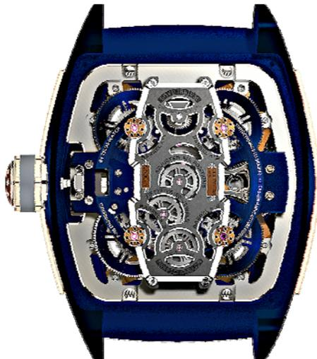
Once again, innovation is part of this particular architecture, to say, that the plate carries only the gear train for the transmission of force to an entire system of flying components, such as, the Tourbillon cages, the minute time bridge and the differential. This set is mounted on 5 ceramic ball bearings and offers an unparalleled reliability ensured by a power reserve of 72 hours.
