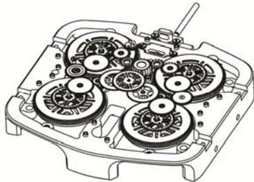
The tourbillons are synchronized (or equilibrated) by a differential device equipped with ceramic ball bearings, which give this set extreme mechanical rigidity, withstanding the impacts and of course the combined torque and mechanical forces from the 4 barrels.
